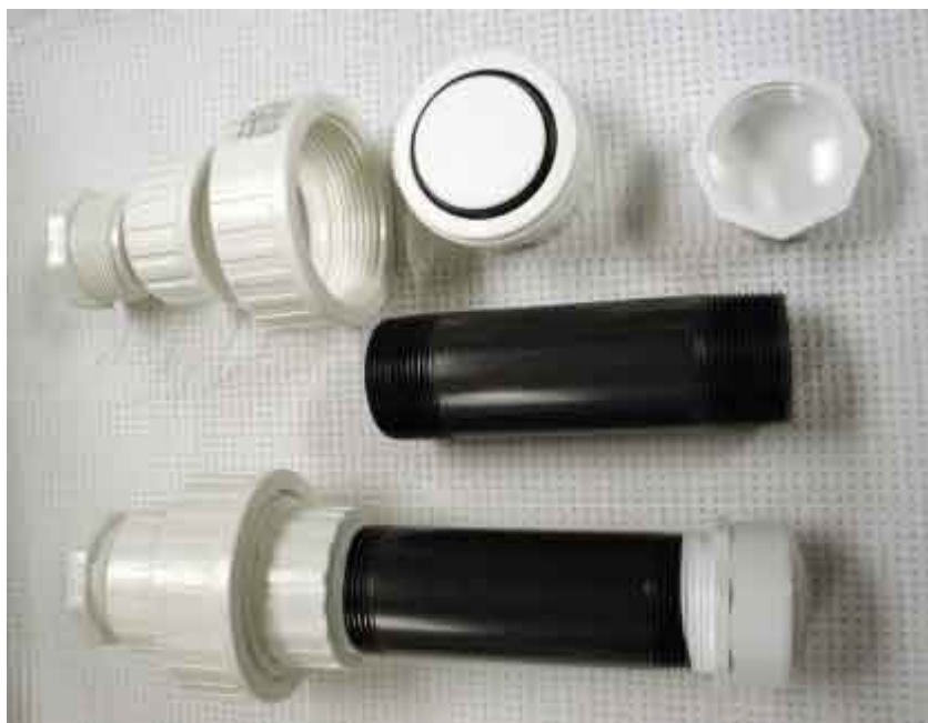
Figure 2.3.2 Optional sample filter holder for DFU. The assembled unit is shown in the bottom of the photograph.
