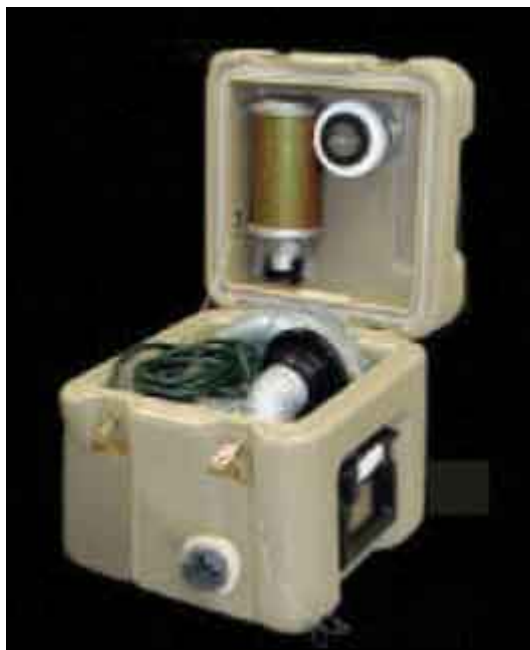
Figure 2.1.1 DFU with lid up to expose the internal pump and filter assembly. The muffer is stored in the lid.
