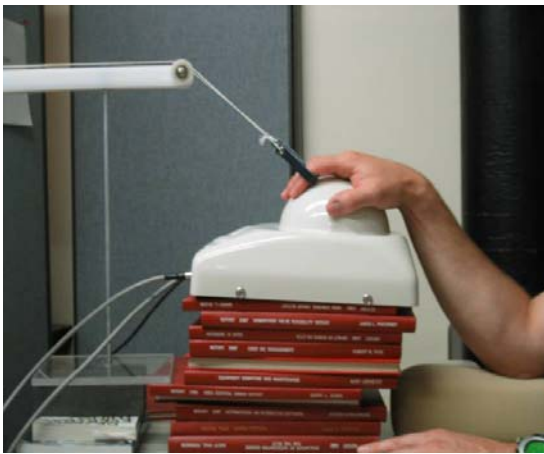
Figure 5. Test C: Wrist flexion with tendon loading
