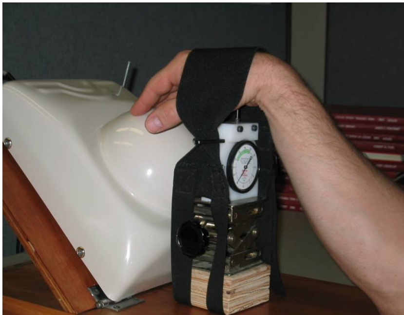
Figure 3. Test B: Wrist flexion with direct pressure
