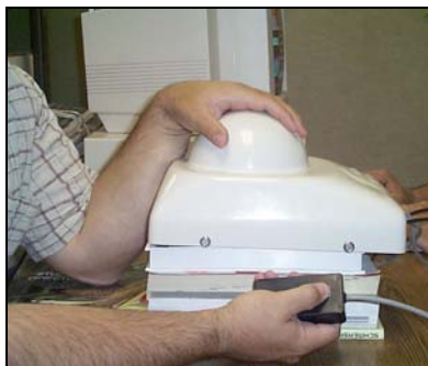
Figure 2. Vibrotactile Testing with Provocative Wrist Posture: 15-minute flexion trial
