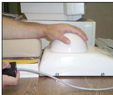
Figure 1. Vibrotactile Testing with Neutral Wrist Posture: Baseline and Post-test
