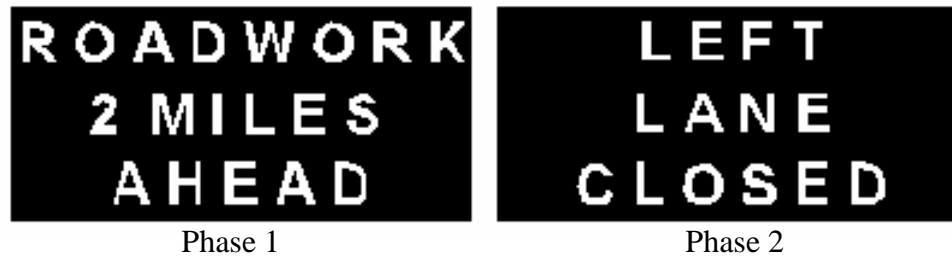
Figure 7. Work Zone Phase Accommodations
