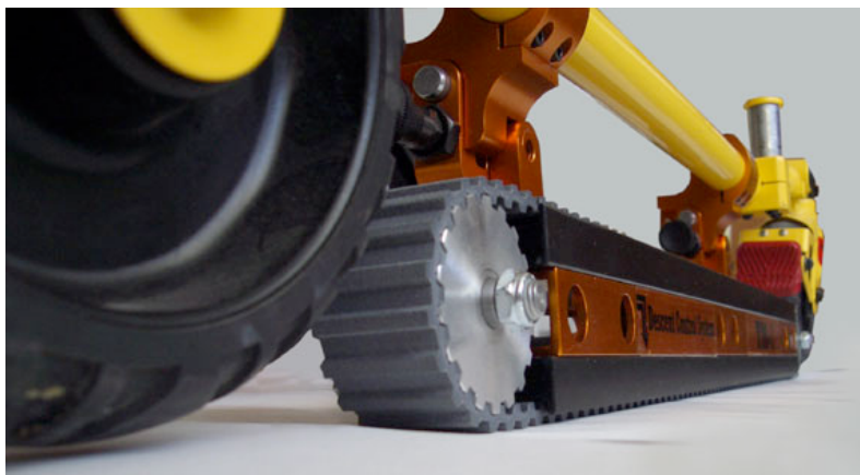
Figure 1. The Descent Control System
