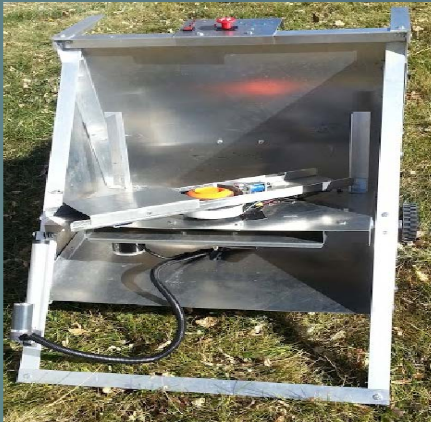
The APT in the testing environment. The Loading mechanism has been detached to better show the launching arm and trigger
