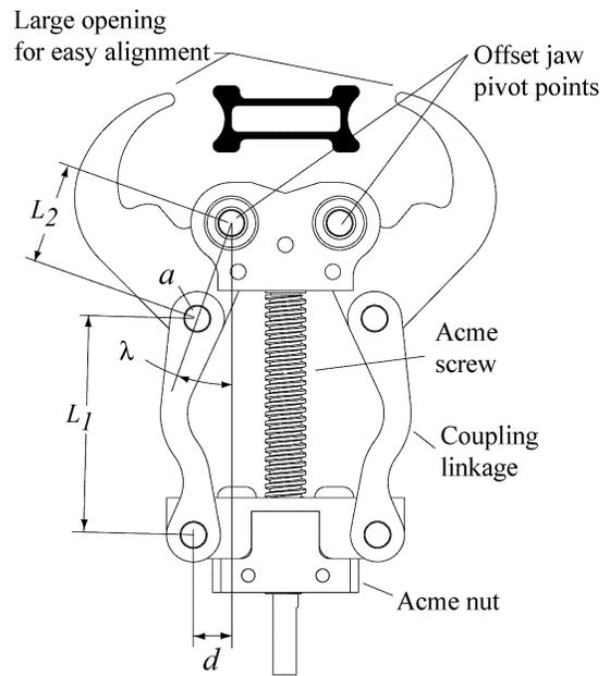
Figure 4. Gripper linkage.
