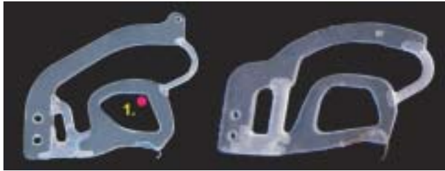
Fig. 12. Photograph of two toe designs that employ overload stops to prevent toe damage. A pin 1 , attached to the robot's foot provides overload protection in conjunction with the hole in each toe surrounding the pin. This ideally causes the toe to disengage upon excessive extension, or in the worst case prevents further extension if the toe does not disengage.
