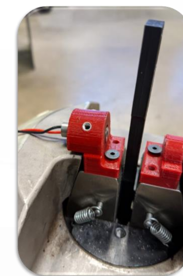
Figure 6. Laser sensor detects when a coupon is centered on the grips within +/- .1 mm
