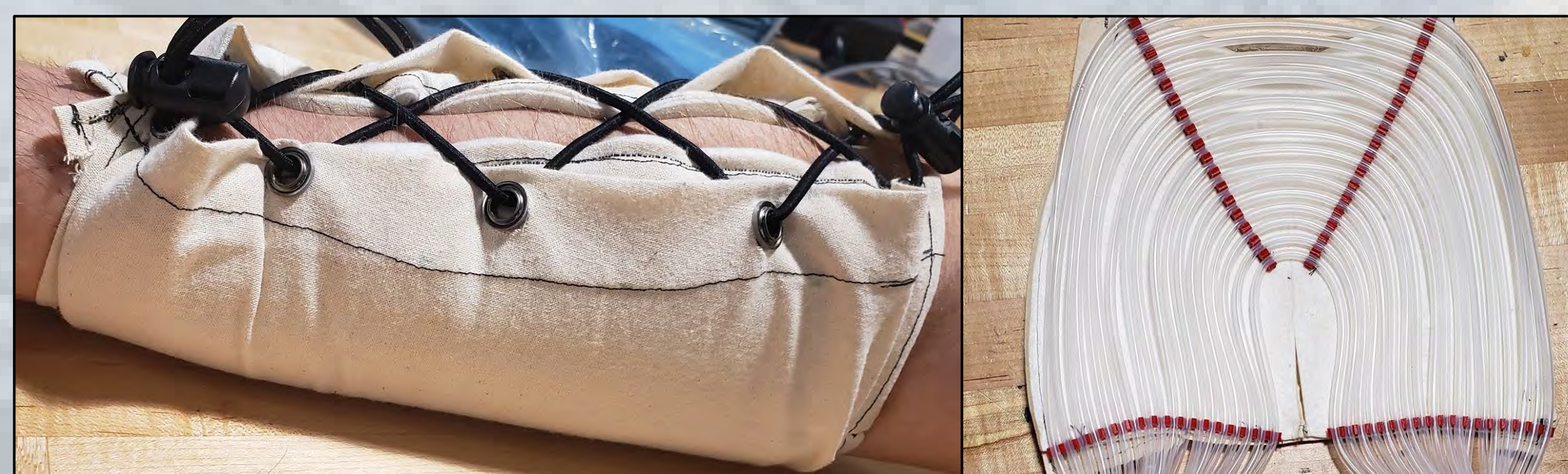
Canvas garment filled with cooling tubes (right), fitted to the forearm with elastic drawstrings woven through grommets (left).
