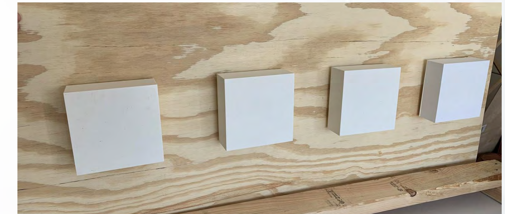
Figure 4: Photo of the bottom side of 3D-printed Helmholtz resonators attached to ½ inch plywood top plate.
