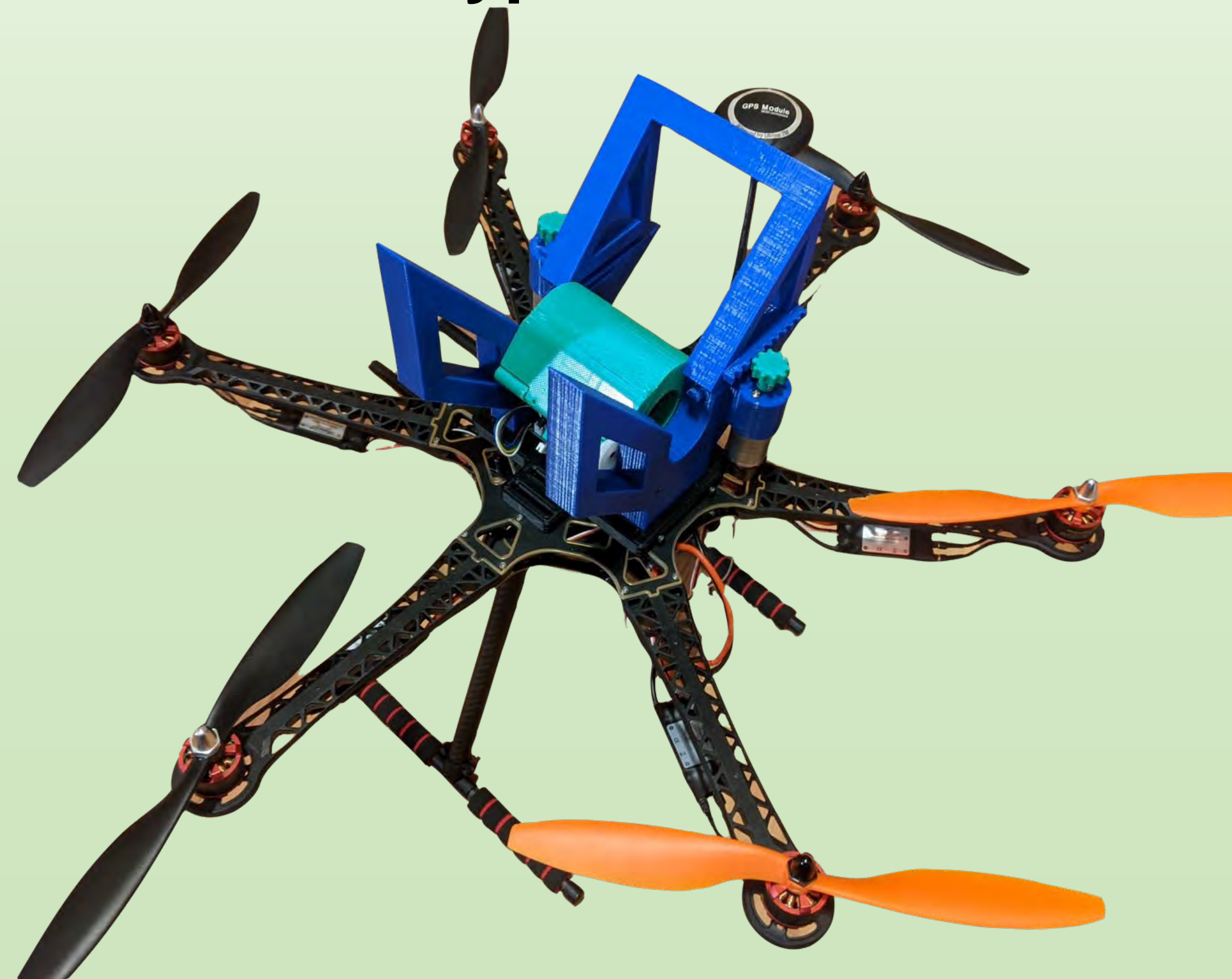
Full Drone Assembly with perching mechanism shown in blue
