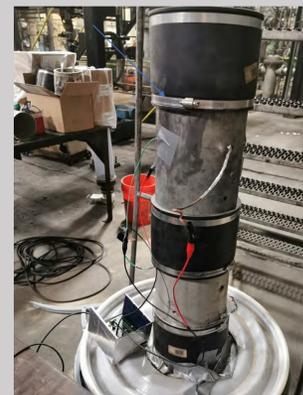
Figure 4: Vertical test assembly with both sensors
