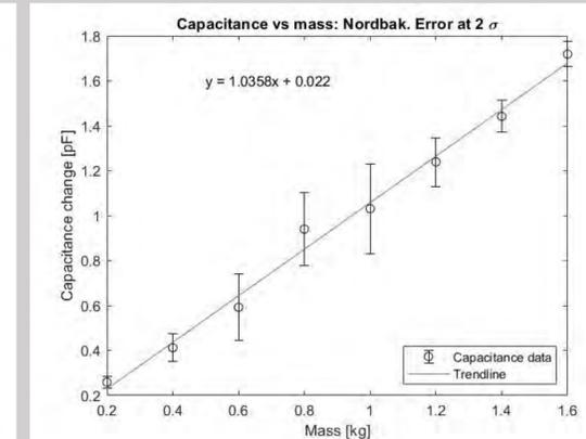
Figure 10: Results of testing varying masses of sand within the Nordbak sensor prototype. While the relationship is still linear, there exists significantly larger standard deviations in this prototype than the hex tile model. Additionally, the slope is significantly greater.
