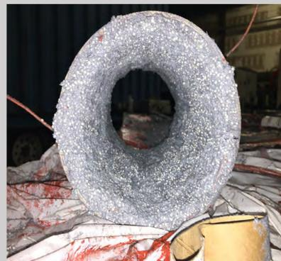
Figure 5: Nordbak Insulator full cover. Nordbak is a 100% solids epoxy that contains ceramic beads to provide abrasion resistance.
