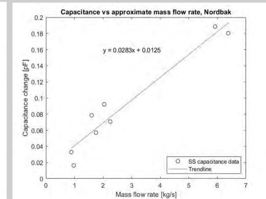
Figure 12: Steady state capacitance data compared to flow rates within the Nordbak prototype. A much stronger linear relationship exists for this model, likely due to experimenters gaining experience at maintaining steady state conditions after the hex tile prototype trials.
