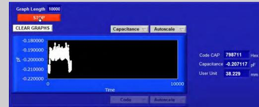
Figure 7: Sensor noise floor
