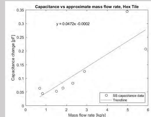
Figure 11: Steady state capacitance data compared to flow rates within the hex tile prototype. As expected, a linear relationship exists under steady state conditions. A high error is present likely due to the difficulty of maintaining steady state conditions at high feed rates.
