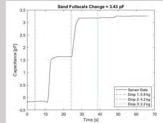
Figure 8: Sensing field was filled incrementally with sand until full to determine full scale output and corresponding mass.
