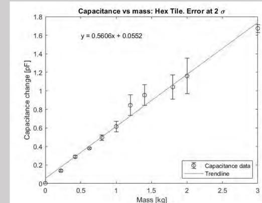
Figure 9: Results of testing varying masses of sand within the hex tile sensor prototype. As expected, the capacitance is linearly correlated to the mass of particulate in the sensing field.
