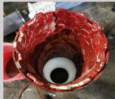
Figure 6: RTV Insulator with tile lining. RTV is room-temperature-vulcanizing silicone that has low shrinkage, no deformation, favorable hardness, and high-temperature, acid, alkali, and ageing resistance.
