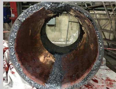
Figure 3: Copper electrodes before insulating layer applied
