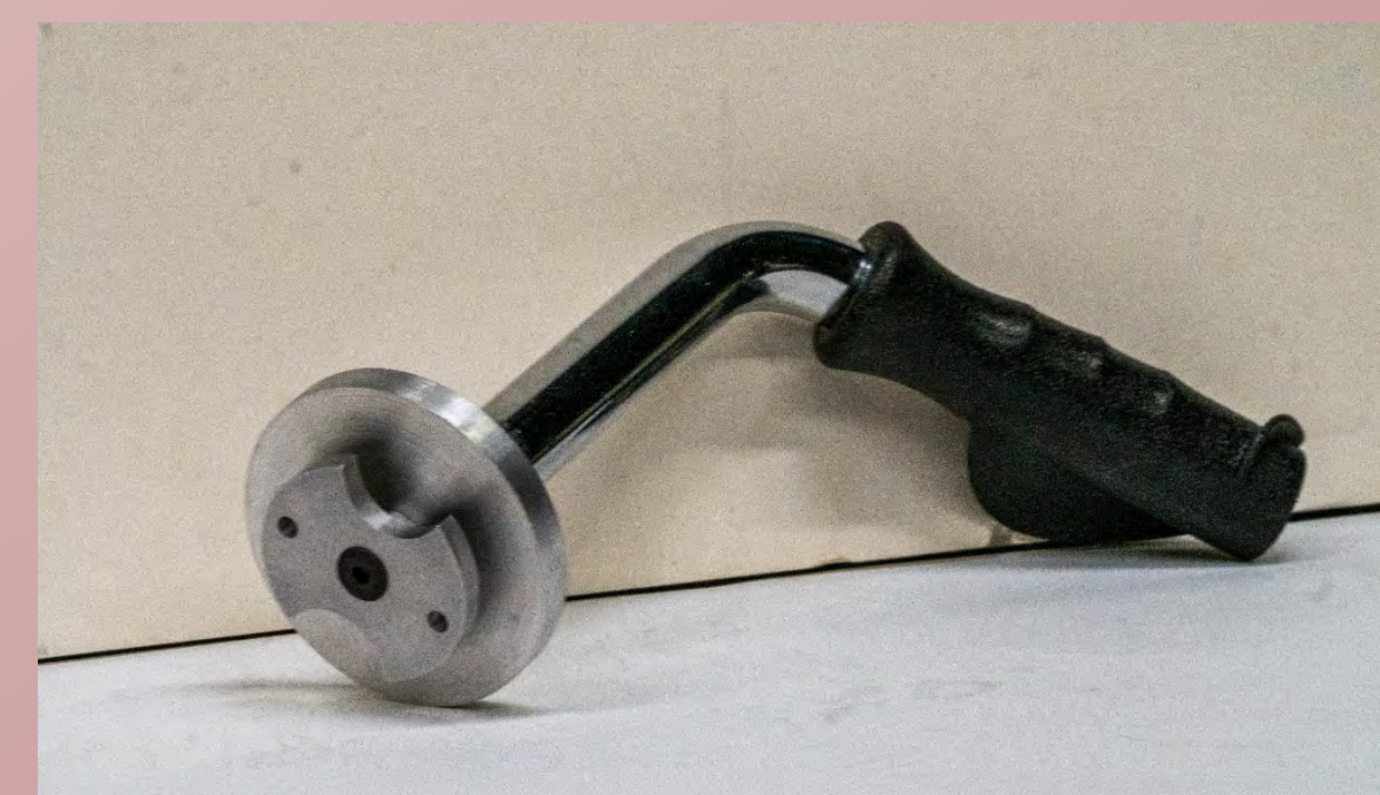
Final manufactured tool changer mounted to walker handle/interface
