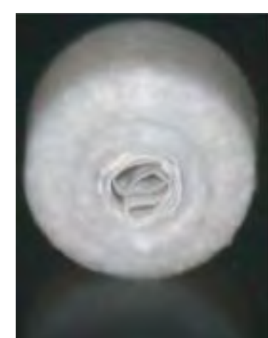
Figure 4 - Completed conduit with electro spun scaffolding inserted into the channel where nerve growth would take place.
