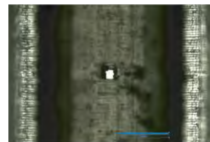
Figure 3 - A magnified picture of the diffusion hole. Microscope was used to measure the size of the diffusion hole. The blue bar represents 1000 micrometers.
