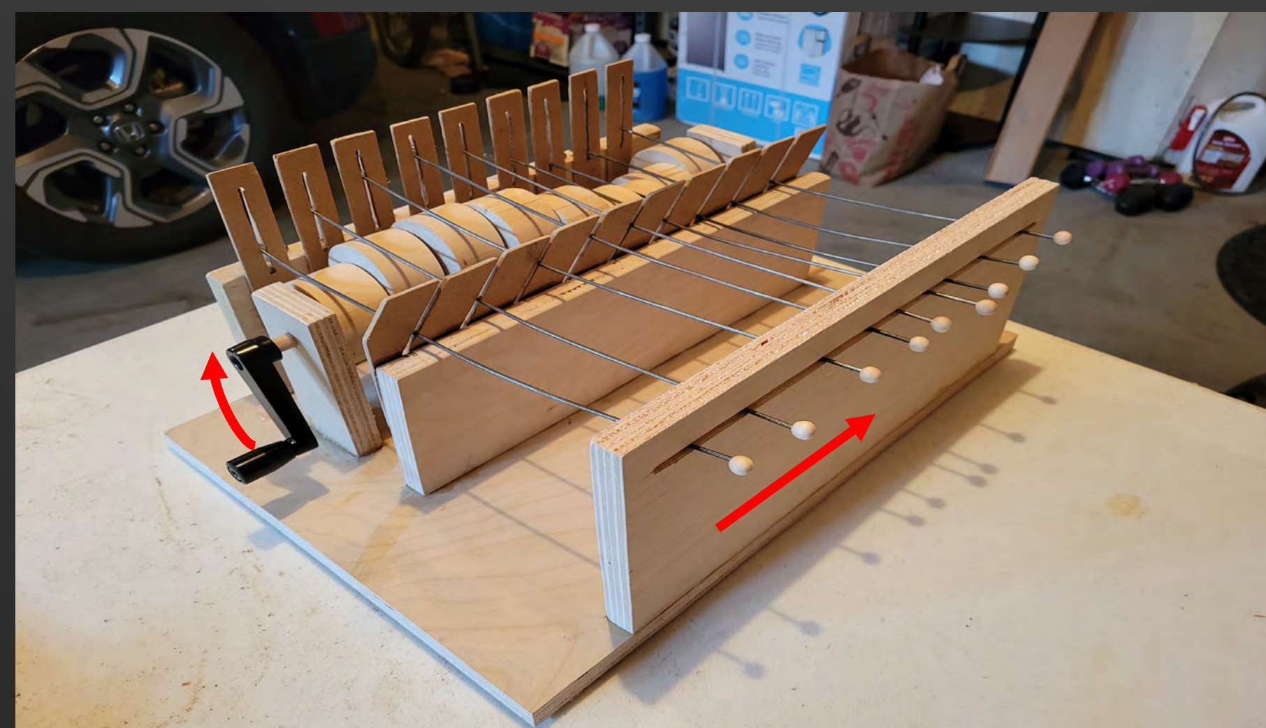
Longitudinal Wave Machine uses a series of mobile balls connected by wire that is driven by a camshaft to create the desired particle trajectory
