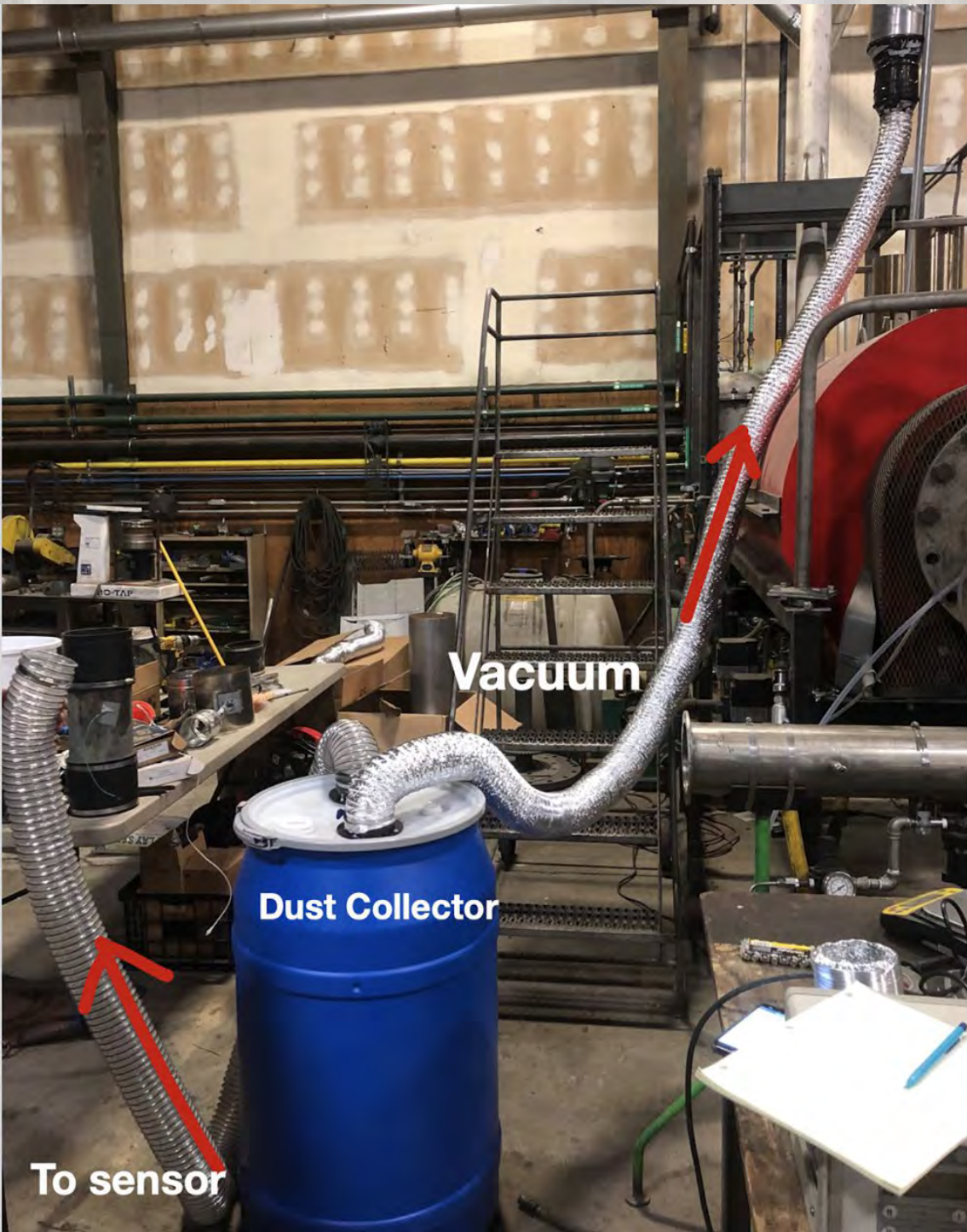
Dust collector shown above. Vacuum pulls material through piping that houses sensor. Material is collected in the blue drum
