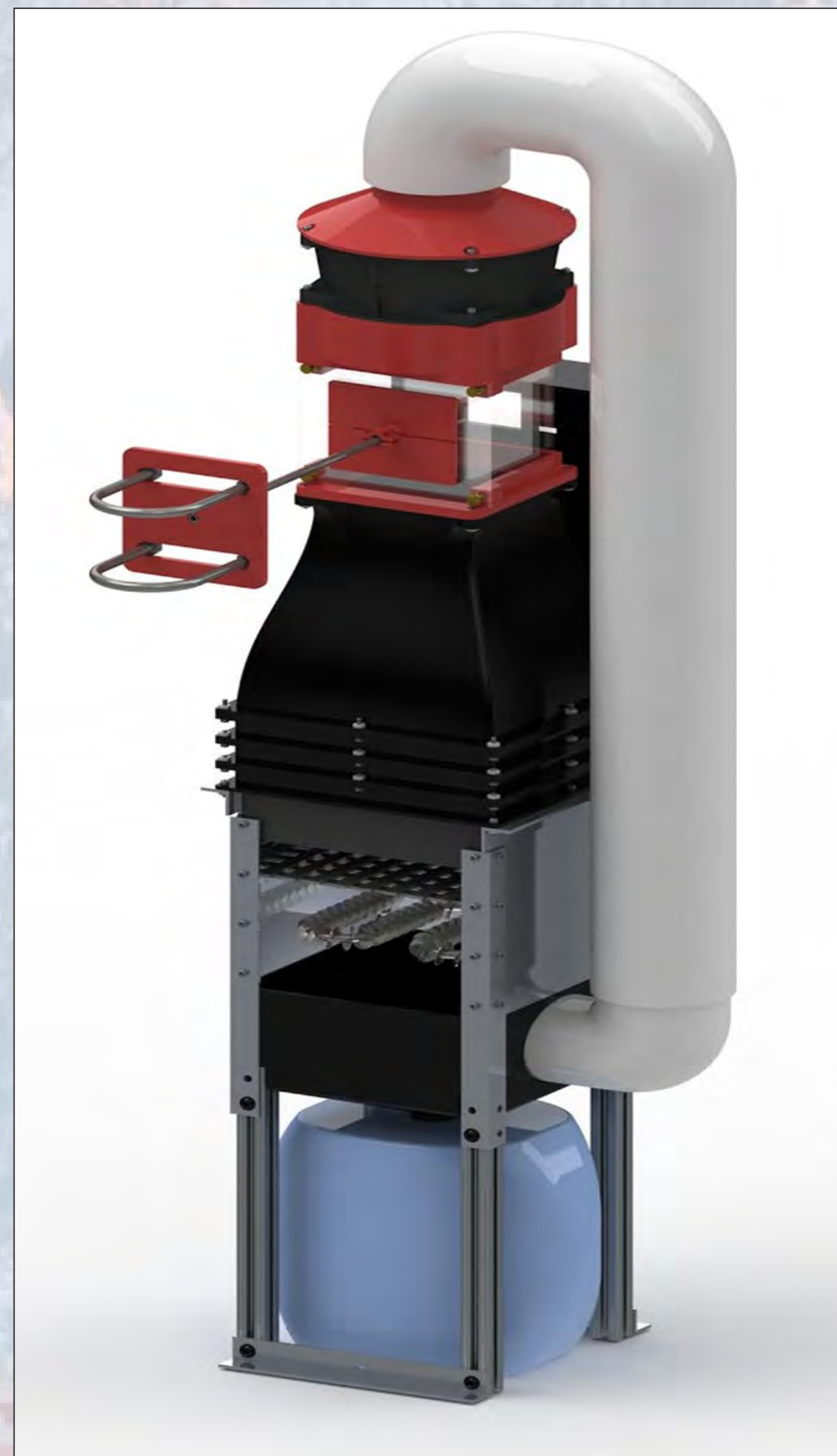
Figure 1. CAD model for closed-loop wind tunnel with heating and humidifier elements.
