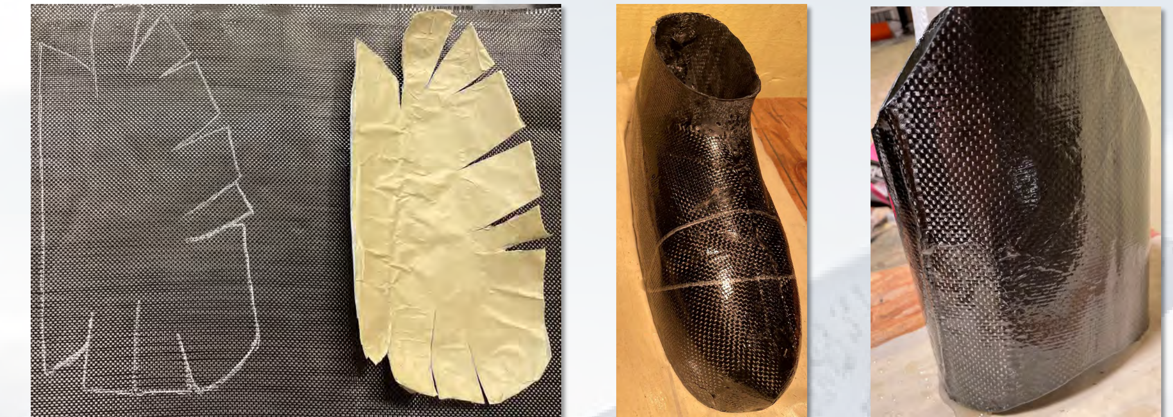
Figure 3: Shell manufacturing process: Cutting carbon fabric to size (left), finished lay up of the lower boot shell (middle), and finished lay up of the upper cuff shell (right).
