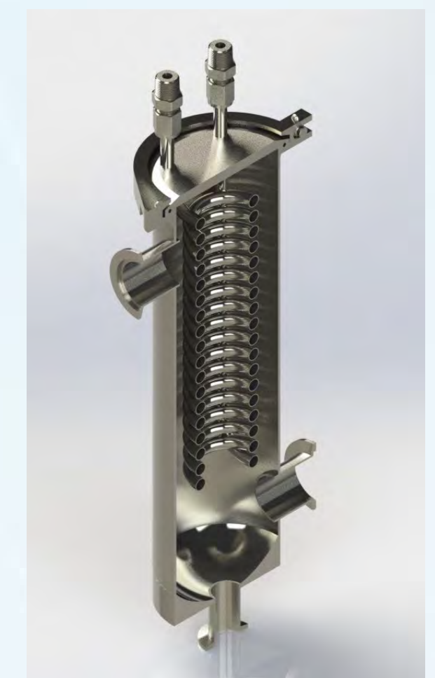
Figure 3: CAD rendering of the final trap design. A steel coil can be seen inserted into the trap to regulate temperature.
