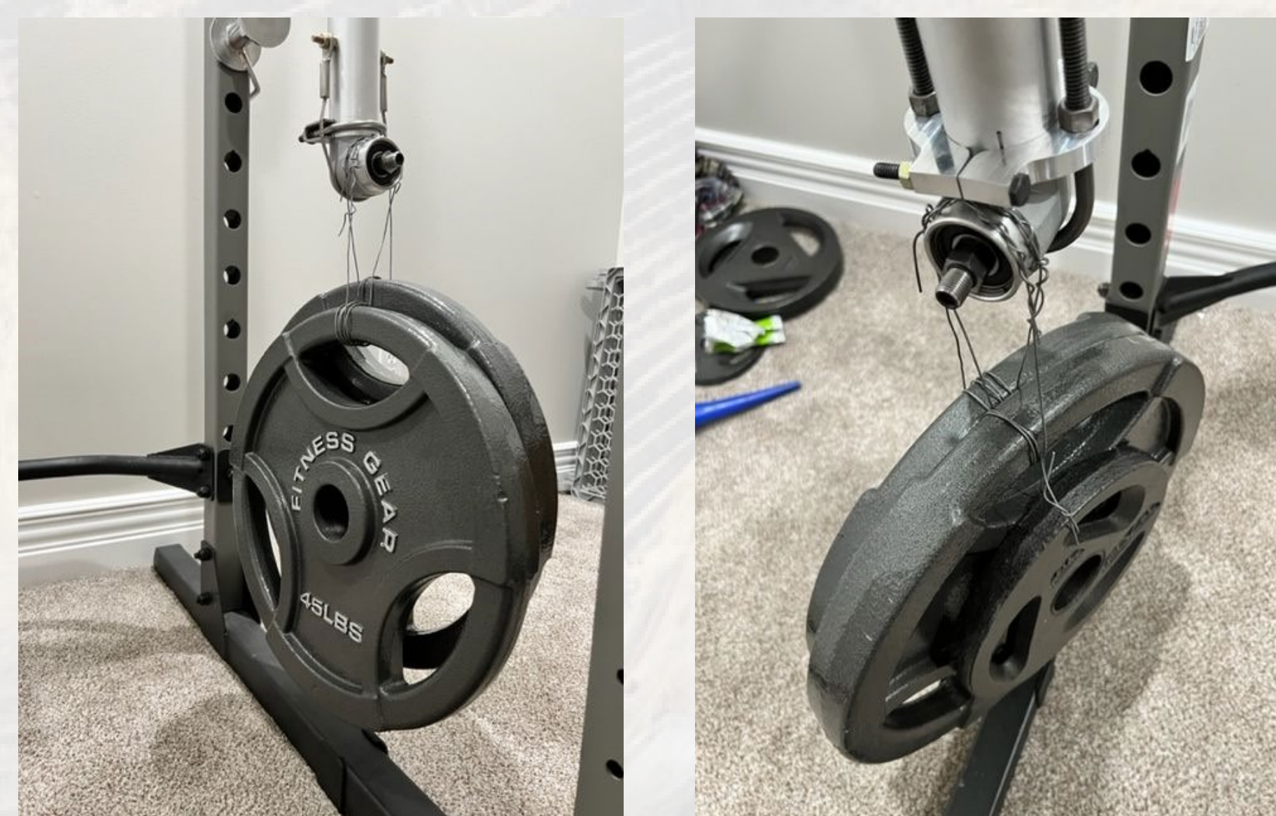
Figure 3: V3 Prototype (left) and V4 Prototype (right) are shown undergoing testing. Both prototypes are holding 45kg using bailing wire.
