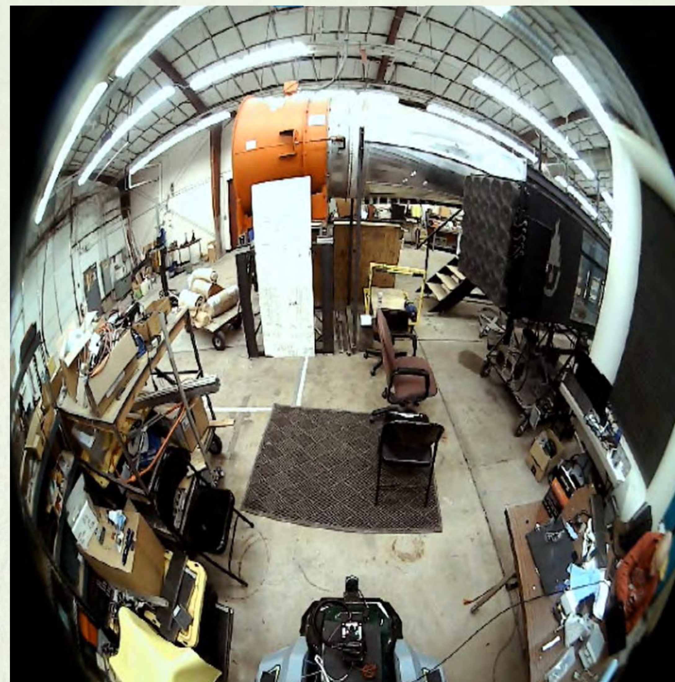
Top-down camera view covering the rear blindspots of the mower. Back of the mower can be seen in the bottom-center of the frame
