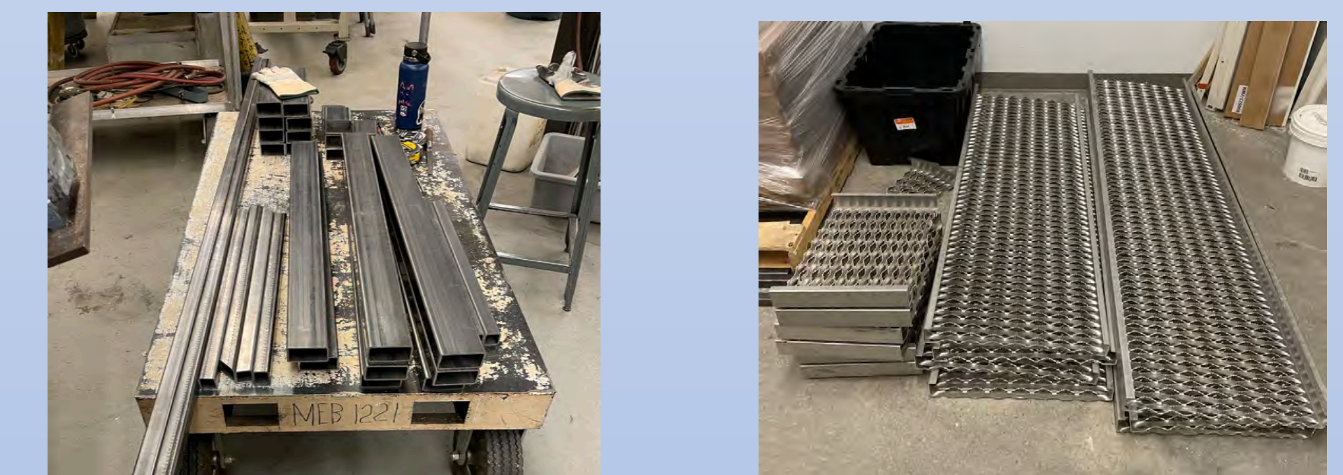
Figure 7: (Left) Steel tubing cut to correct lengths for the platform. (Right), Aluminum grip-strut planks being bolted together.
