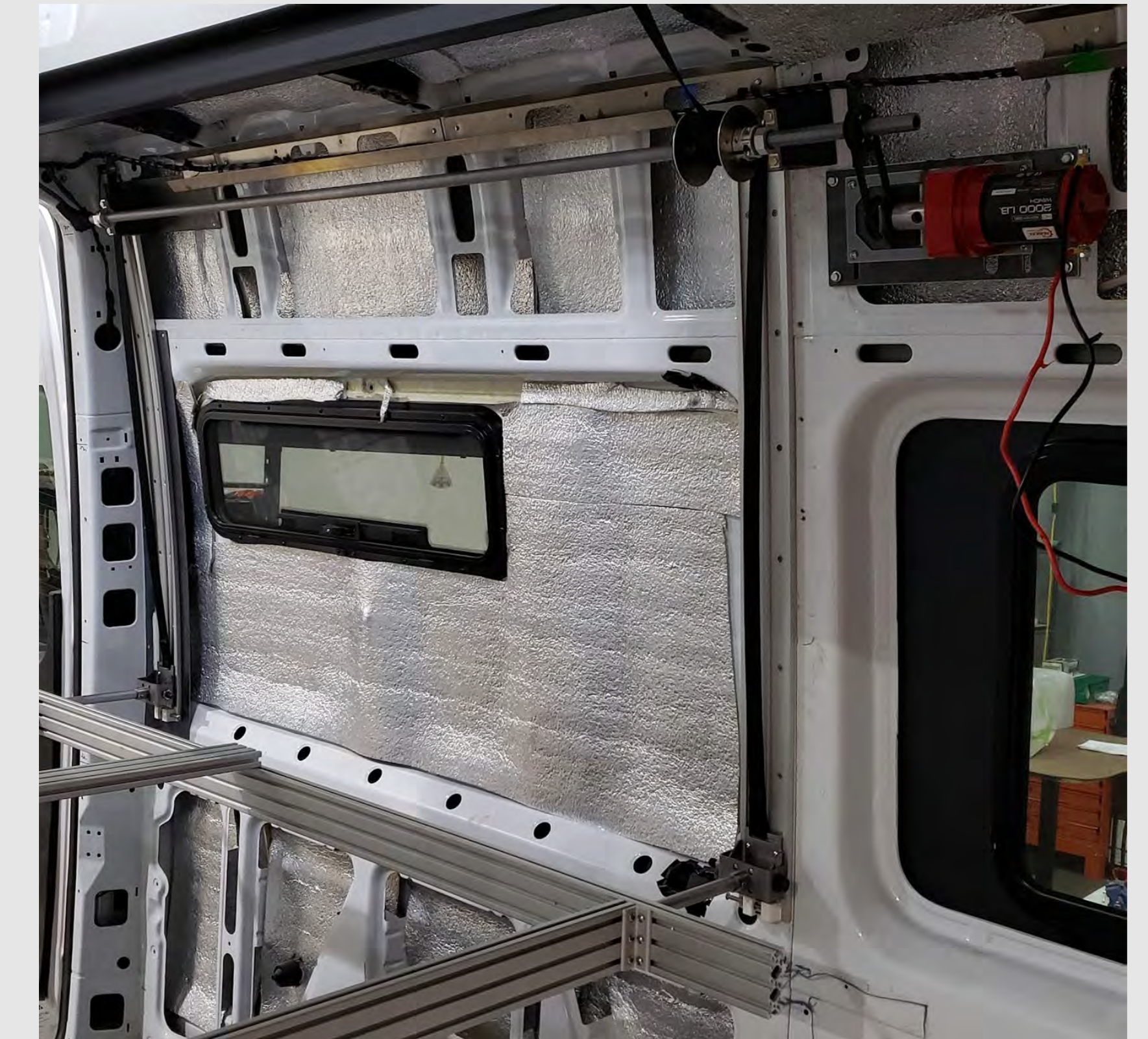
Figure 6: Lift bed frame attached to wall with spooling system
