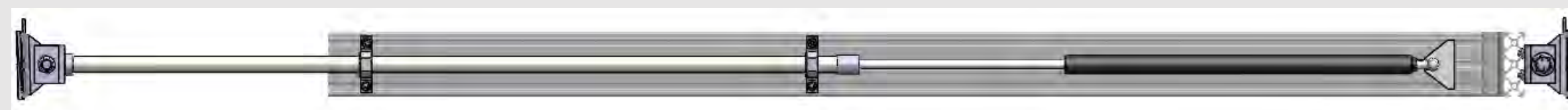
Figure 4: Retracting arms attached to the frame that adjust for van wall curvature
