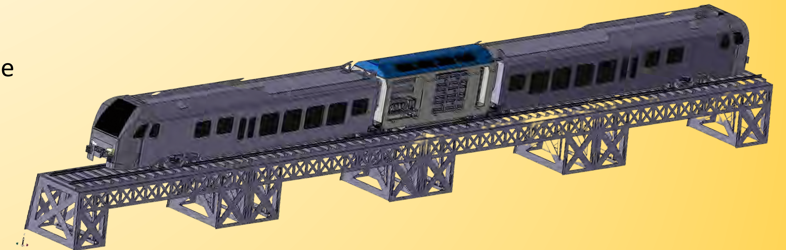
Figure 4: Full train assembly, including front and rear passenger train and "power pack" car
