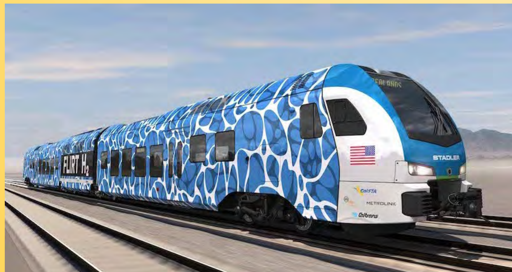
Figure 1: Stadler's FLIRT H 2 production train with passenger train car on either side of "Power Pack" car
