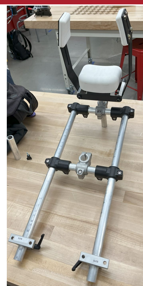
Figure 3: Assembled Headrest and U-Bar
