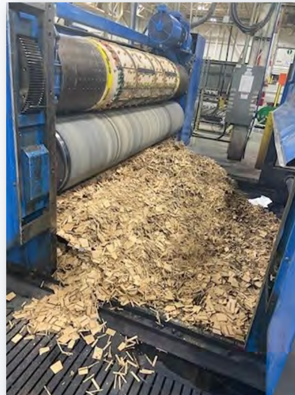
Figure 1: Scrap buildup in the rear of the Ward Flexo 329
