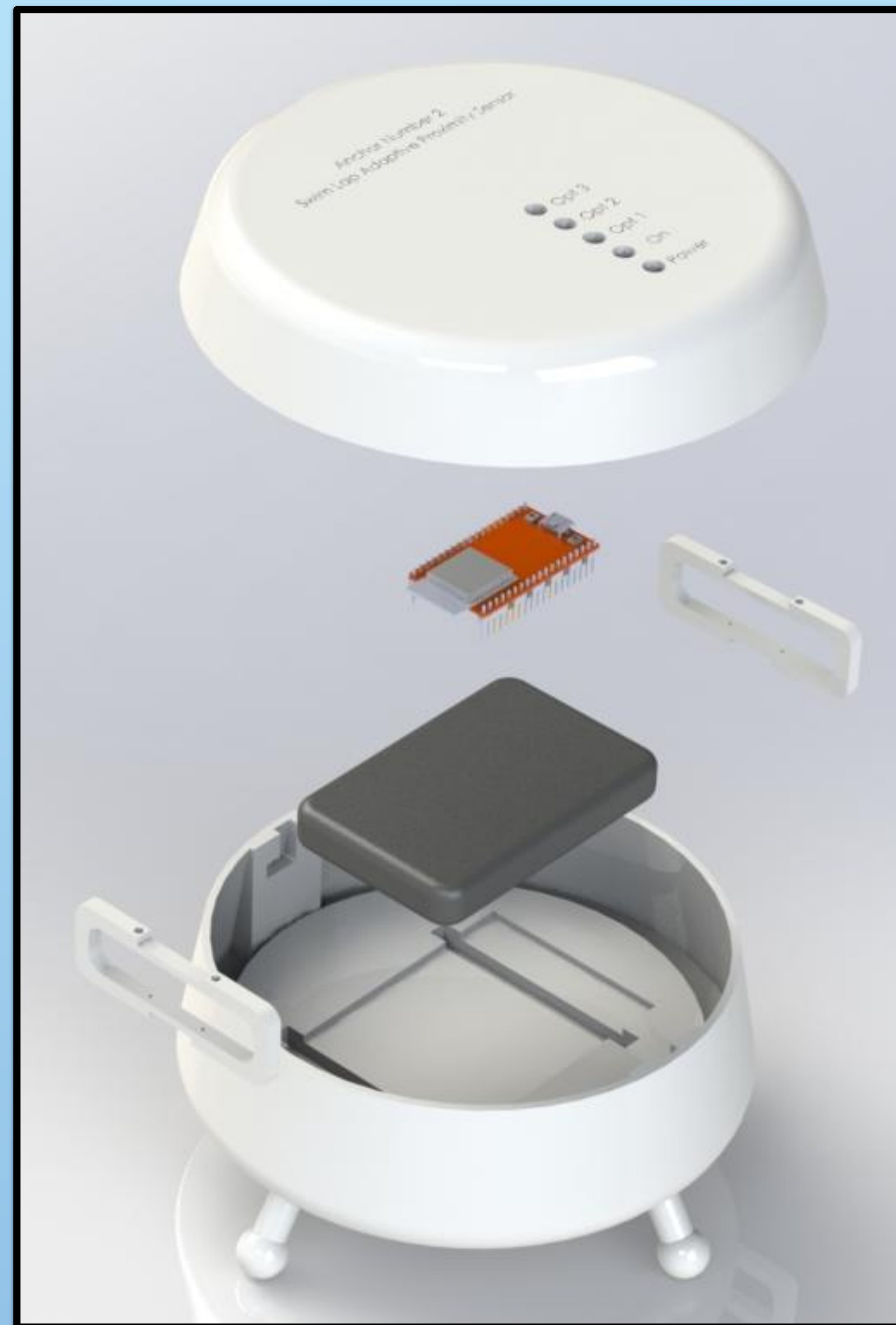
A rendering of the model of one of the anchors used for triangulation of the swimmer. The white parts show the waterproof casing. The black box is the battery. The red microcontroller is an ESP32 UWB Pro.
