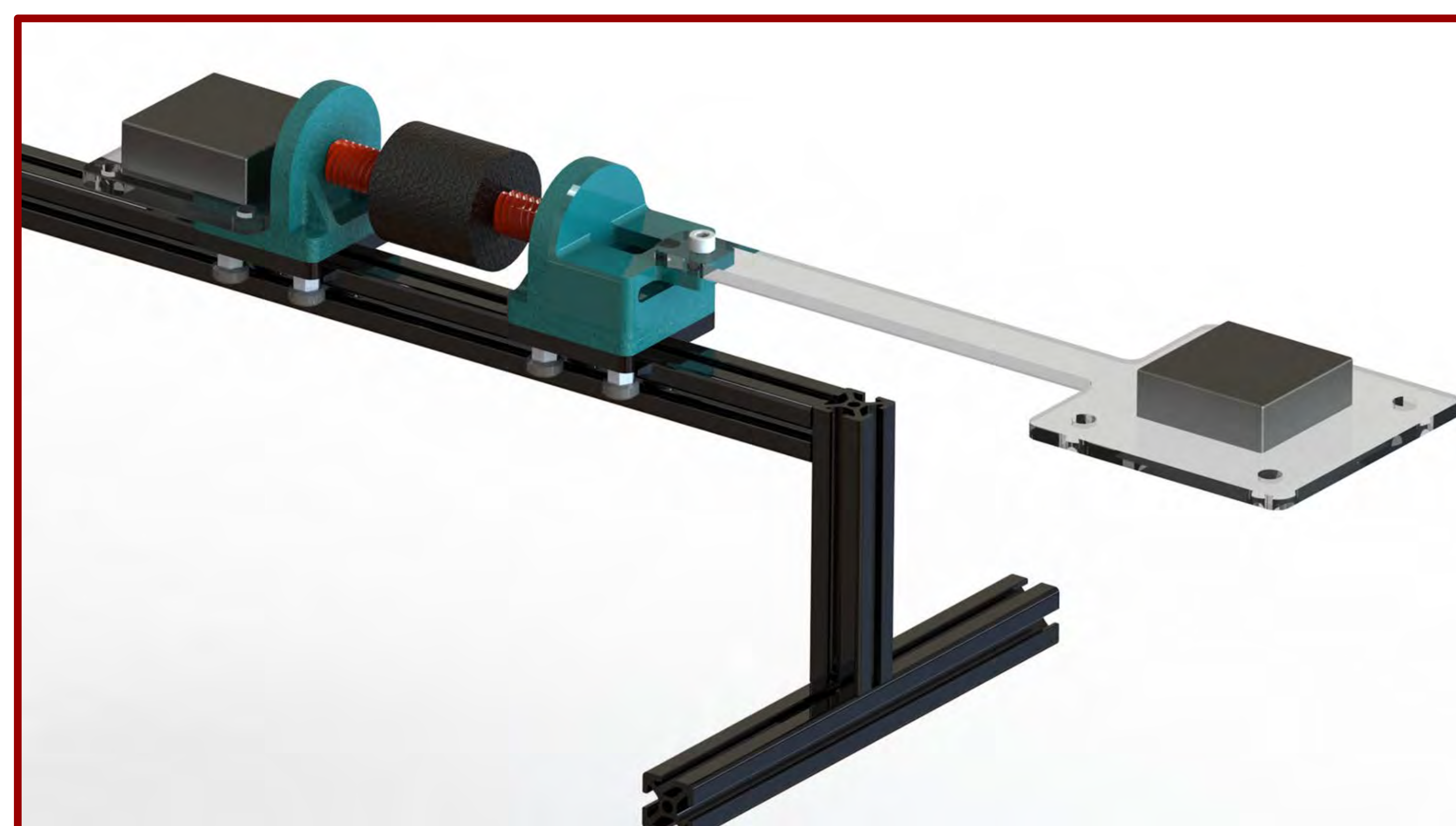
Figure 3: Rendering of the testing set up. Includes the rail system and accelerometer connection points.
