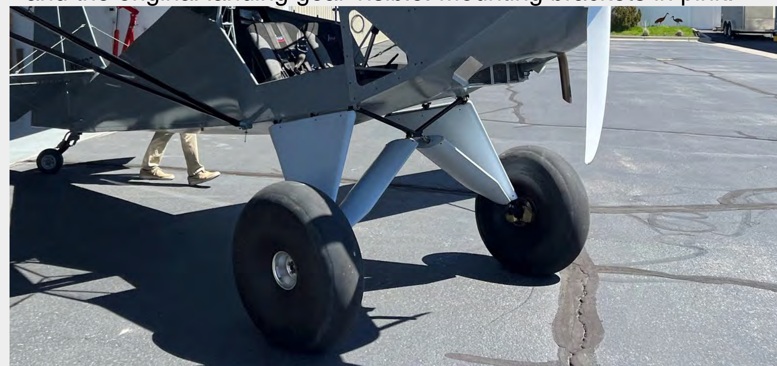
Figure 5: Experimental aircraft with designed fairings attached
