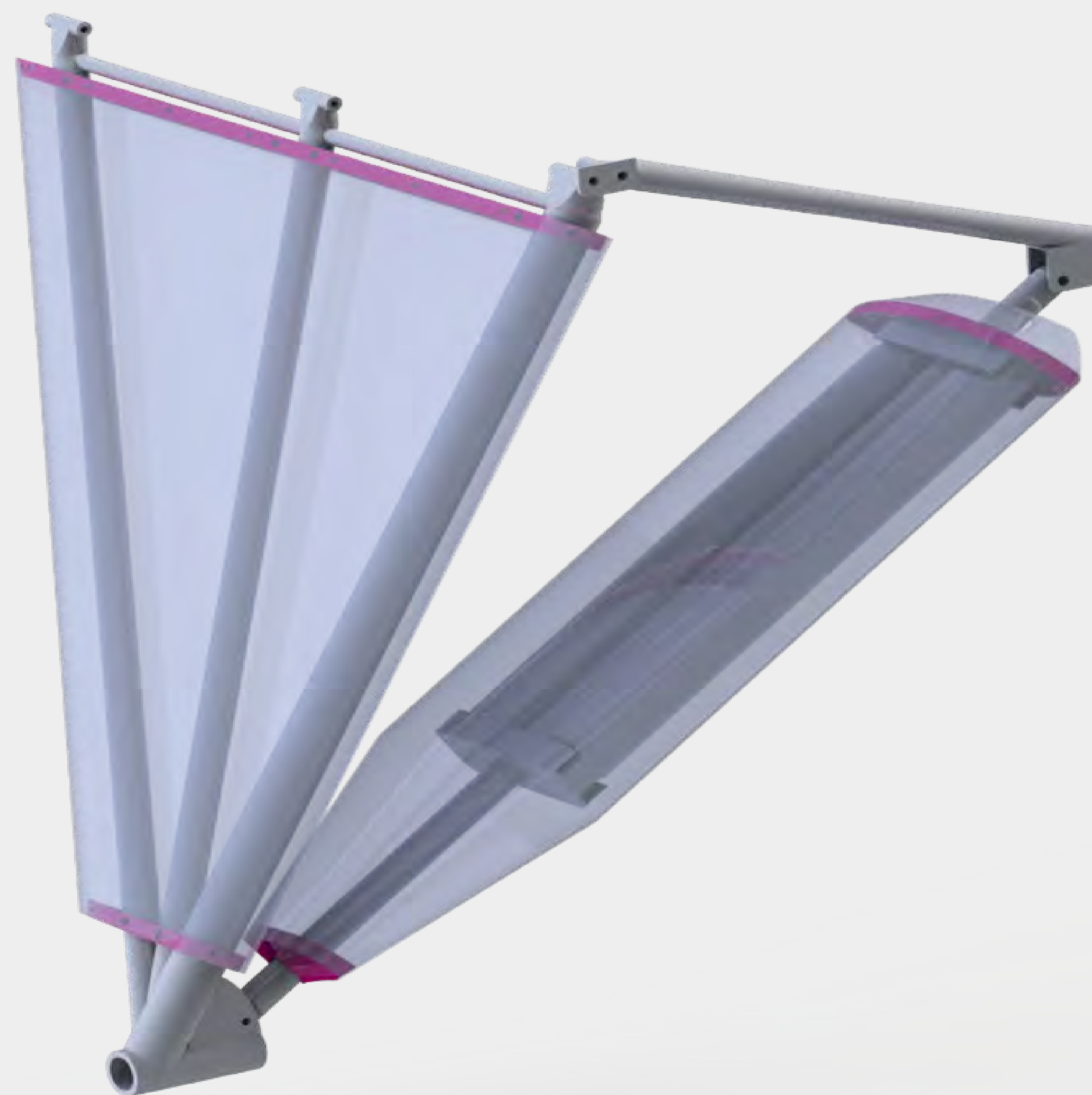
Figure 4: CAD image of the designed fairings (transparent parts) and the original landing gear visible. Mounting brackets in pink.
