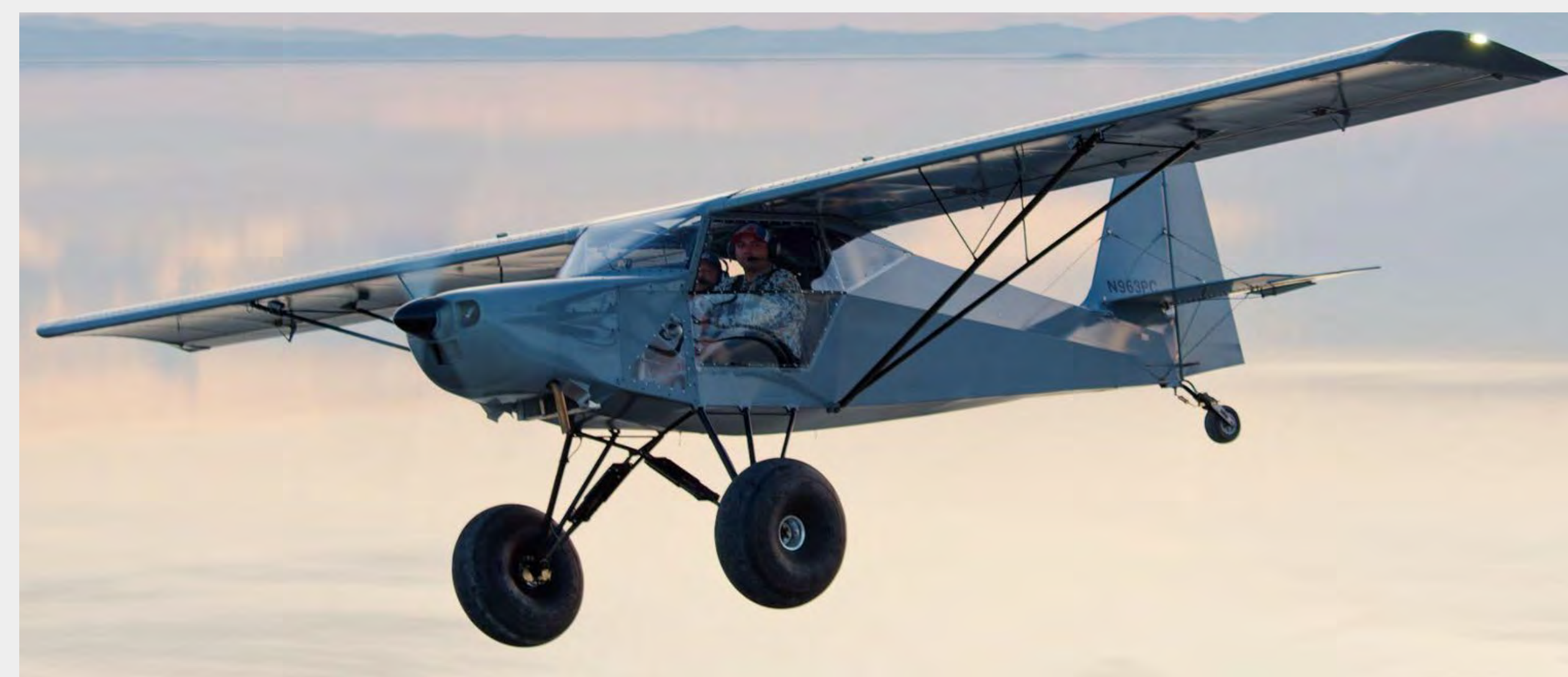
Figure 3: Experimental aircraft with uncovered landing gear
