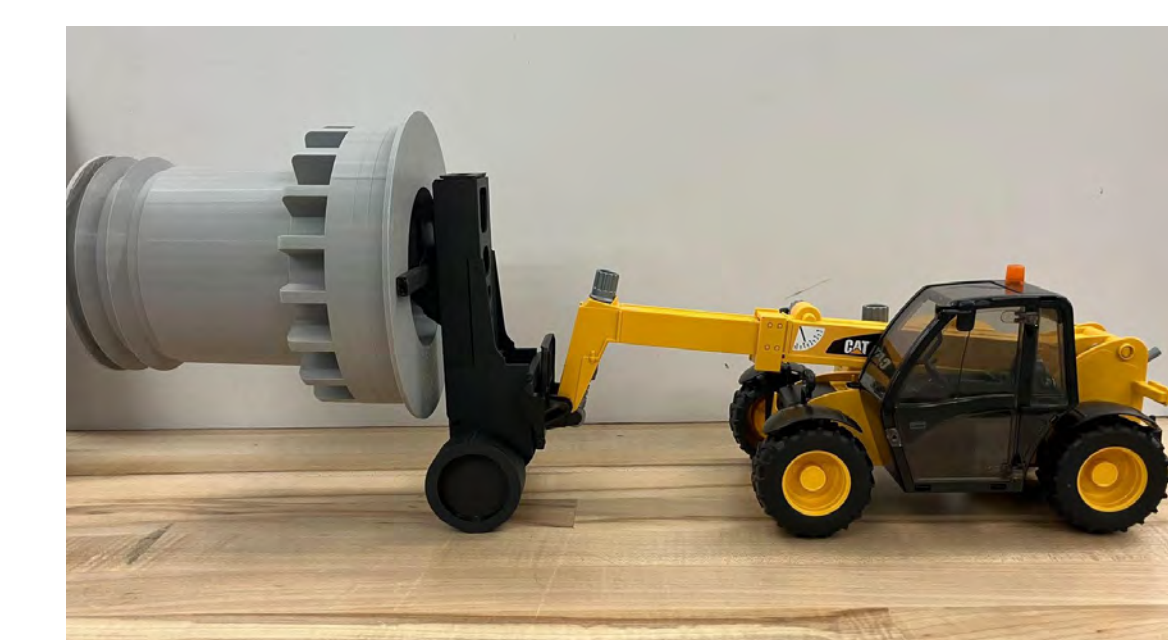
Figure 8: Picture of 3D printed device holding a 3D printed cone at a 16:1 scale, attached to 16:1 scaled CAT toy.
