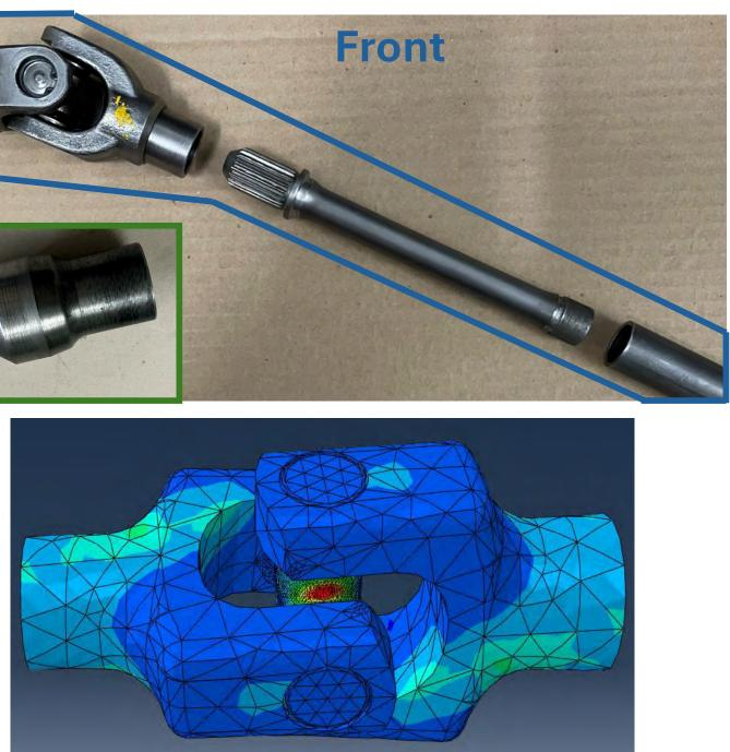
Based on a worst-case scenario where the engine stalls at full speed. Applying a 1355 N\*m torque on the driveshaft. The max stress of 2.625 kPa is far below the yield stress of 420000 kPa (420 MPa) for AISI 4340 Steel.
