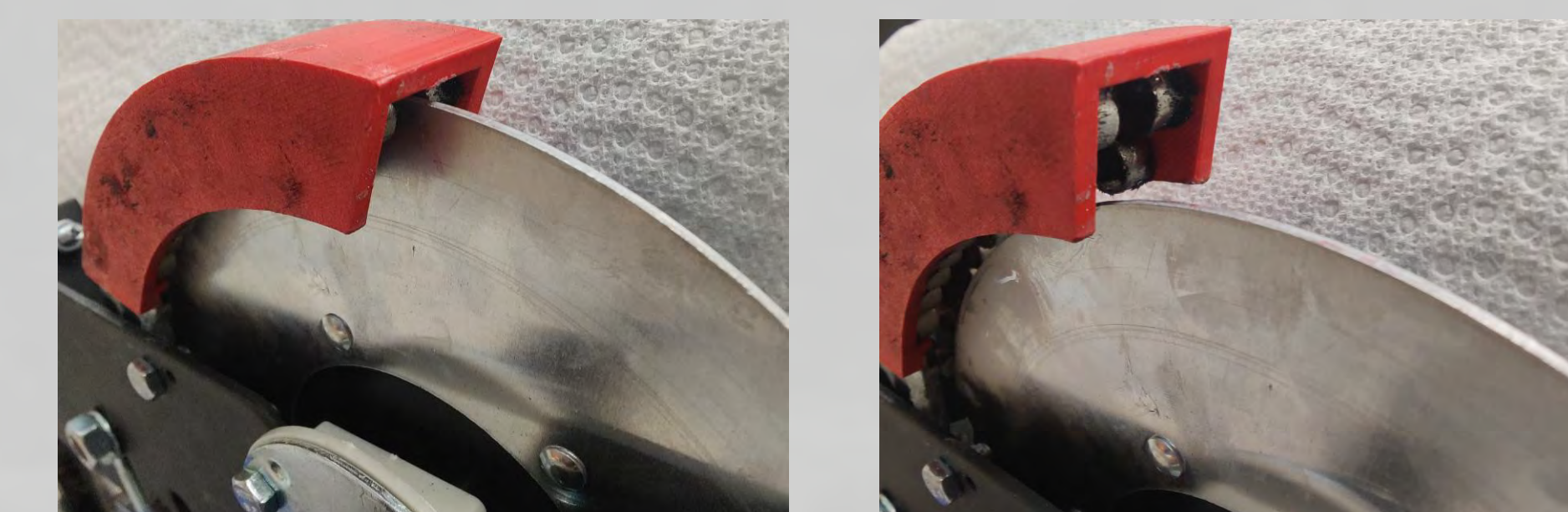
Full magnet overlap with high resistance is shown on the left and no magnet overlap with low resistance is shown on the right.
