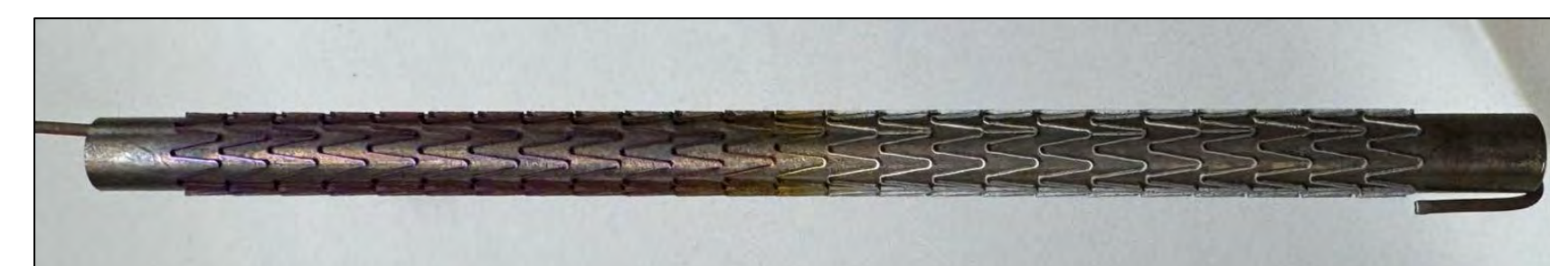
Fig. 8: A laser cut stent, loaded onto a stainless steel tube, half heated.
