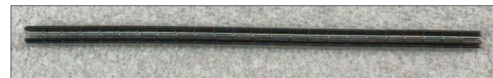
Fig. 7: A laser cut stent, after being deburred and acid etched.
