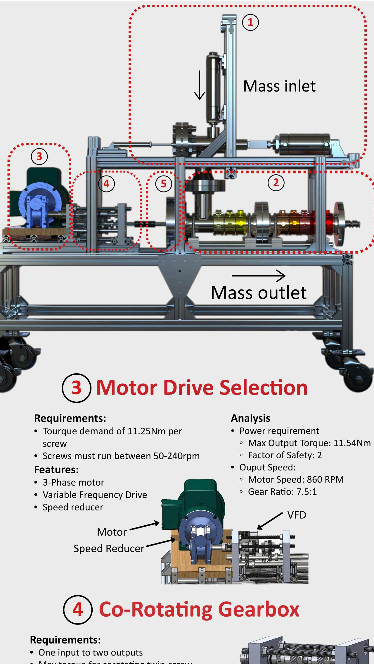
• Max torque for corotating twin-screw is 26.7 Nm per screw
