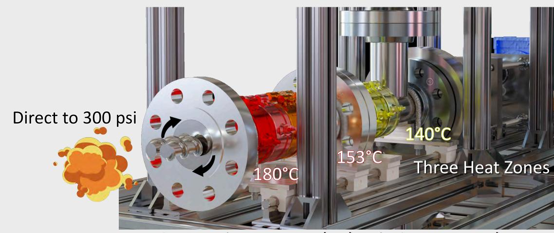
**Co-Rotating Intermeshed Twin Screw Extruder**
