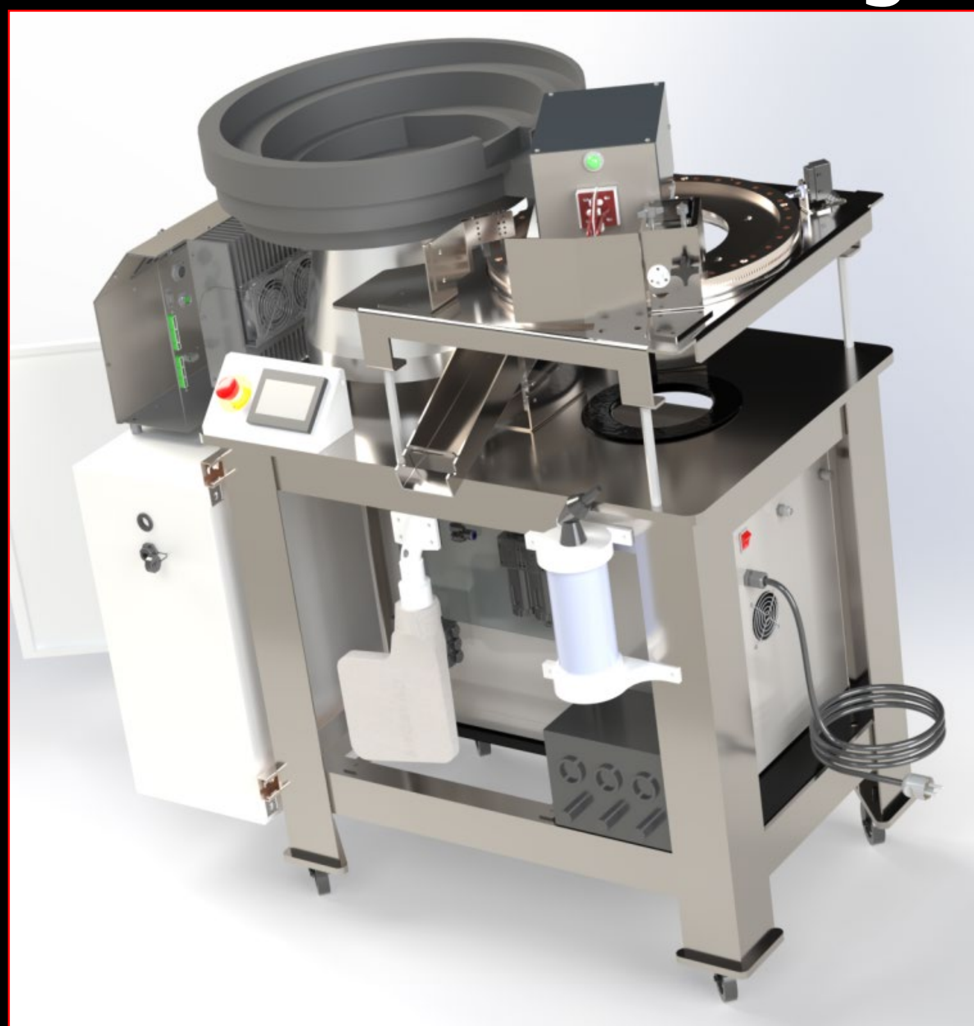
Figure 1. CAD model of the fully integrated broadhead assembly device, illustrating the complete configuration of the vibratory bowl, induction heater, and the pneumatic subsystem consisting of a nylon sprayer and a vacuum.
