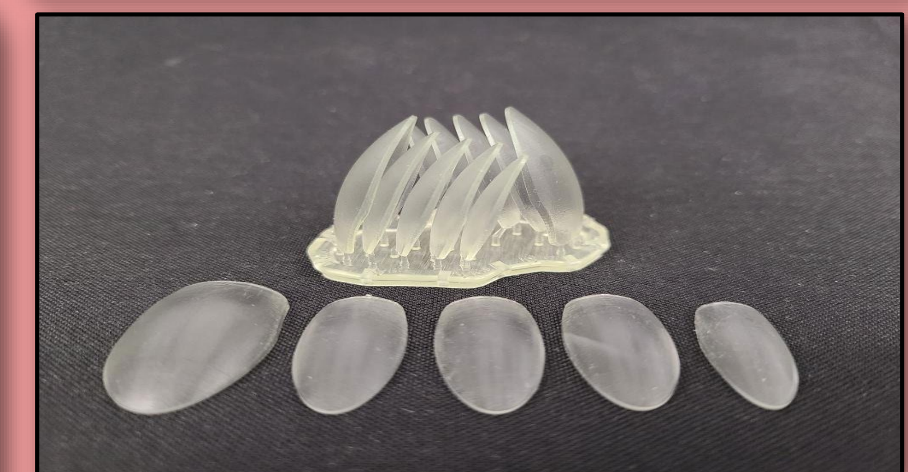
Figure 5. Resin-printed set of 10 nails in clear resin, shown after printing, washing, and curing.
