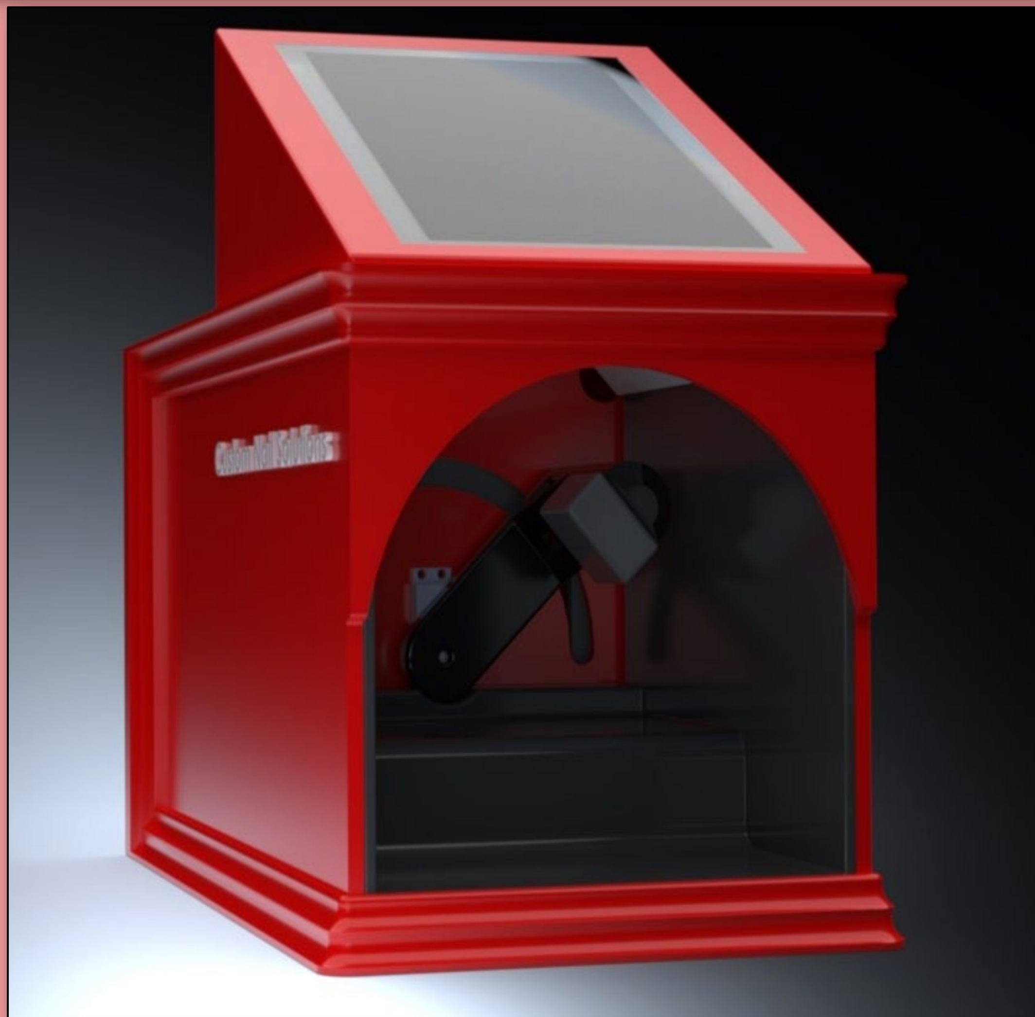
Figure 1. Hand-scanning enclosure featuring the user hand port, motorized camera arm, and onboard touchscreen interface.
